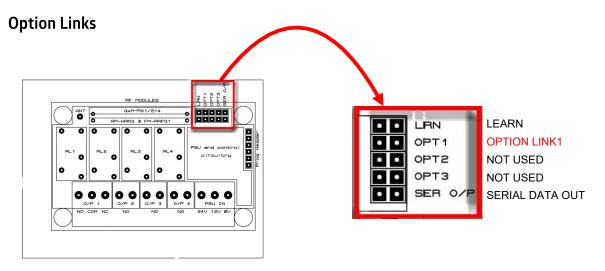
The action of the relay outputs is set by the Option link setting Jumper. A link is made / removed by the small shorting link 'cap' placed over the pin header.
