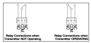
Please Note: The relay contacts in this unit are for functional use only and must not be used for power isolation purposes
