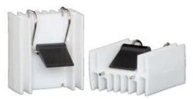
The unique design (patent pending) of the WC Series heat sinks combines a tin plated, solderable, integral cam clip with an compressed ceramic heat sink body for an all-in-one solution to through-hole mounting of TO-220, TO-247, and TO-264 packages. These self-aligning heat sinks feature solderable feet and an integrated clip with 13.2 (lbf) of force on the center of the device to enhance thermal performance.
