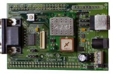
The EZURiO Development Kit is designed to support the rapid development of hardware, applications and software for the EZURiO range of BISM II Bluetooth Intelligent Serial Modules and WISM Wireless LAN modules. The EZURiO development kit is available in five options to cover the widest range of wireless technologies, including hardware support for development of applications for the Siemens MC55 GSM GPRS modules.
