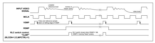
Figure 10 Reset Level Clamp Operation (CLAMPCTRL=1), non-CDS mode only
