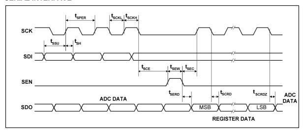
Figure 4 Serial Interface Timing
