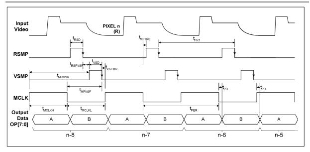
Figure 3 Single-channel CDS Input Video Timing
