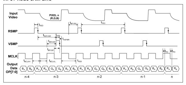
Figure 1 Three-channel CDS Input Video Timing
