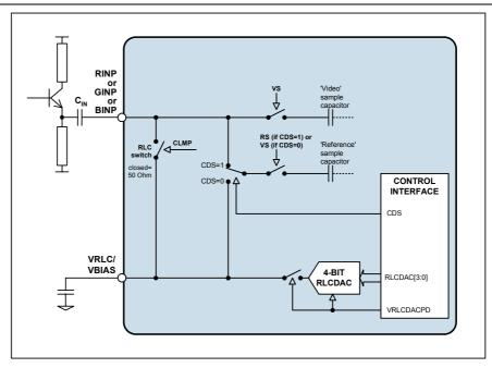
Figure 12 CDS/non-CDS Input Configuration
