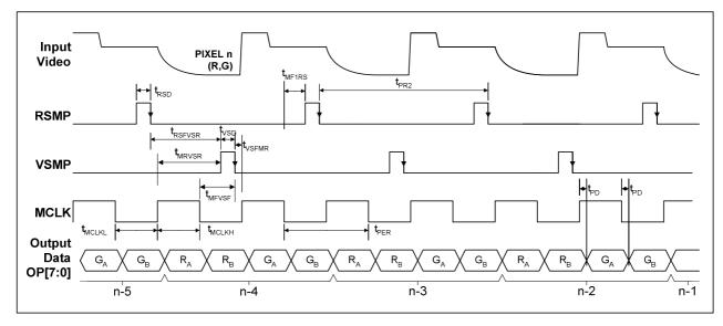
Figure 2 Two-channel CDS Input Video Timing
