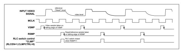
Figure 9 Reset Level Clamp Operation (CLAMPCTRL=0), CDS operation shown, non-CDS also possible
