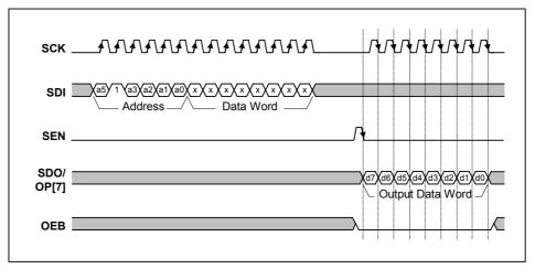
Figure 19 Serial Interface Register Read-back
