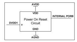
Figure 5 Internal Power On Reset Circuit Schematic
