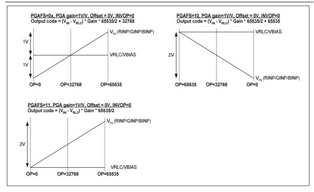
Figure 15 ADC Input Black Level Adjust Settings
