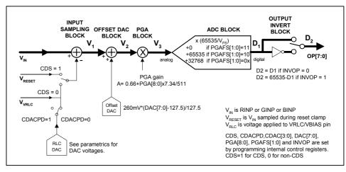
Figure 16 Overall Signal Flow
