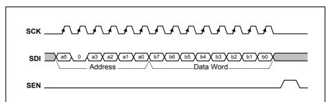
Figure 18 Serial Interface Register Write
