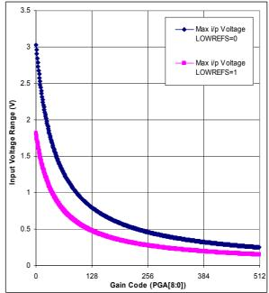
Figure 13 PGA Gain Characteristic
