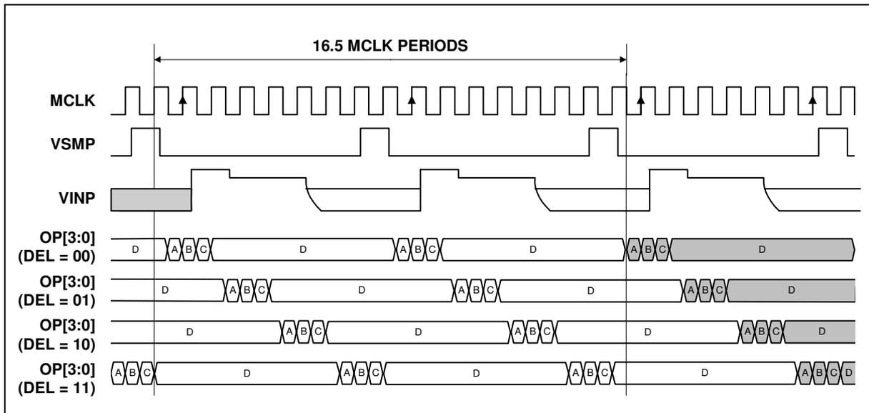
Figure 17 Mode 4 Operation (MCLK:VSMP Ratio = 8:1)
