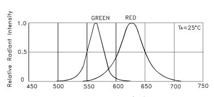
wavelength  $\times$  (nm) RELATIVE INTENSITY Vs. WAVELENGTH
