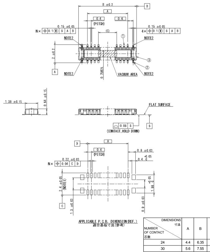
Note 1) Dimension  $3.9 \pm 0.05$  is recommended in case repair is needed.
