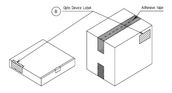
Type A Material / box : Cardboard C5BF Type B,C Material / box : Cardoard K5AF Partition : Cardoard K5BF
