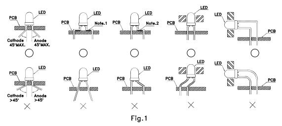
"() " Correct mounting method "imes" Incorrect mounting method
