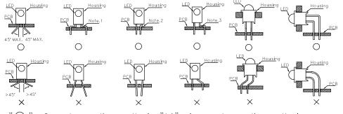
"○" Correct mounting method "×" Incorrect mounting method Note 1-3: Do not route PCB trace in the contact area between the leadframe and the PCB to prevent short-circuits.
