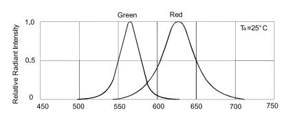
$wavelength \ \lambda(nm)$  Relative Intensity Vs. Wavelength
