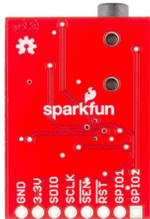
Underside of breakout board showing pin labels
