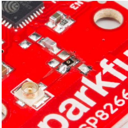
An (ugly, uncleaned) resistor swapped from printed antenna to U.FL antenna.
