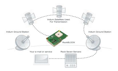
The RockBLOCK allows you to send and receive short messages from anywhere on Earth with a clear view of the sky. It works far beyond the reach of WiFi and GSM networks.
