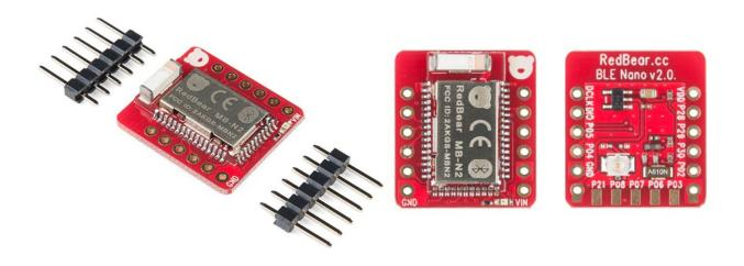
The BLE Nano v2 from RedBearLab is one of the smallest Bluetooth 4.2/5.0 Low Energy (BLE) development boards in the market. At each BLE Nano's core is a Nordic nRF52832, an ARM Cortex-M4F SoC plus BLE capable of running at 64MHz with ultra low power consumption. The RedBearLab BLE Nano v2 also supports numerous different wireless devices running iOS 7/8, Android 4.3 or higher, and Windows Phone 8.1.
