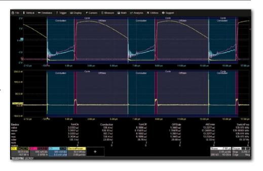
errors and the measurement parameters provide details of single cycle or average device power losses. Beyond the advanced power loss measurement capabilities, the Power Analyzer modulation analysis capabilities provide insight to understand control loop response to critical events such as a power supply's soft start performance or step response to line and load changes.
