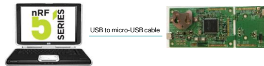
Figure 12 Configuration for application development with nRF52 SDK
