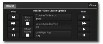
Search through long records of decoded data by entering specific message or frame details.
