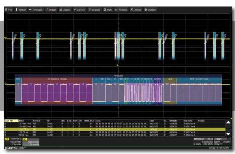
With CAN and CAN FD trigger and decode the oscilloscope becomes the ideal tool for debugging CAN controllers, busses and systems. Identify and isolate specific frames with ID, Remote and Error frame triggering. Decoding CAN signals provides tremendous insight into activity on the bus, and measurement tools enable fast analysis of bus performance.
