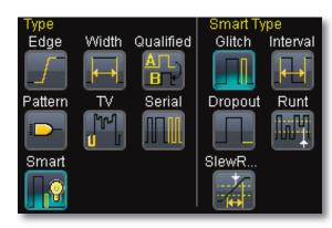
The advanced triggering of the MSO Xs-A goes well beyond the basic edge trigger and digital pattern trigger that many MSOs offer. Advanced triggers like runt and dropout and slew rate help find abnormal signals. The Qualified AB trigger can be used to connect multiple trigger events together.
