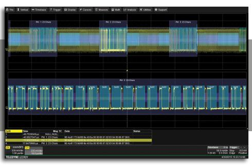
The SpaceWire decode adds a unique set of tools to your Teledyne LeCroy oscilloscope that simplifies the design, debug, and maintenance of SpaceWire systems. The high speed SpaceWire data stream is annotated directly on the physical layer waveforms. Various sections of the protocol are color-coded to make it easy to understand the protocol traffic. The decoder provides an interactive table, search, and zoom to make debugging fast and effective.
