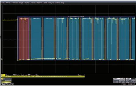
Color-coded overlaid protocol decode makes it easy to understand your serial data messages.
