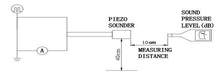
In the measuring test, buzzer is placed as follows:
