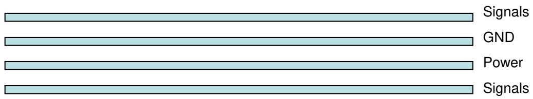
Figure 8: Typical 4-layer PCB construction
