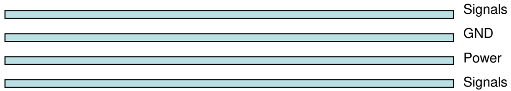
Figure 17: Typical 4-layer PCB construction
