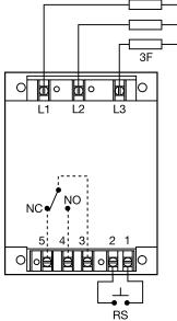
F = Fuses NO = Normally Open NC = Normally Closed RS = Optional Remote Reset Switch
