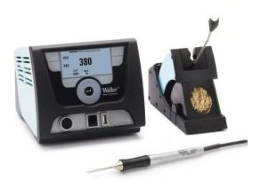
WX 1 control unit with WXMP Micro soldering pencil (40W / 12V) and WDH 50 safety rest
