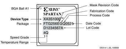
Figure 2: Spartan-3 BGA Package Marking Example for Part Number XA3S1000-4 FTG256Q
