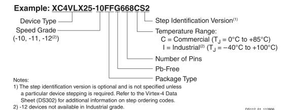
Figure 1: Virtex-4 FPGA Ordering Information
