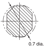
XC5E DIP terminal cross-section view
