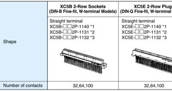
\*1: Terminal type/ Straight, 4mm \*2: Terminal type/ Straight, 13mm \*3: Terminal type/ Straight, 17mm
