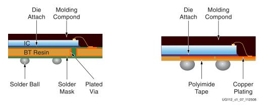
Figure 1-7: Rigid BT-Based Substrate Chip Scale Packages, Left; Flex-Based Tape Substrate, Right
