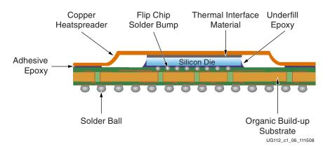
Figure 1-6: Flip-Chip BGA Package with Type II Lid
