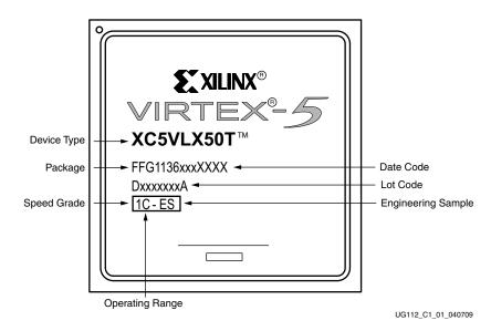
Figure 1-1: Top Marking (for Large Device Packages)
