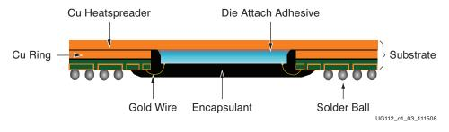
Figure 1-3: Cavity-Down BGA Package
