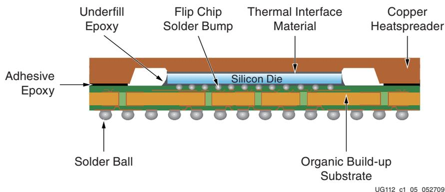
Figure 1-5: Flip-Chip BGA Package with Type I Lid
