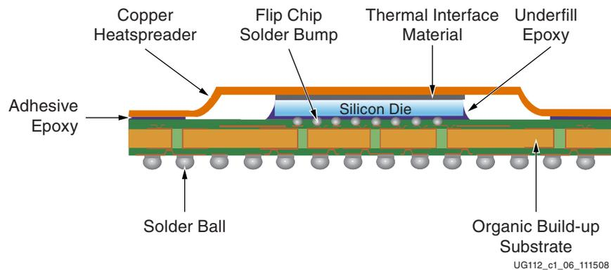
Figure 1-6: Flip-Chip BGA Package with Type II Lid
