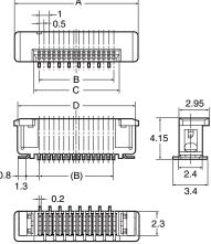
Printed Circuit Board Matching Dimensions (Top View)
