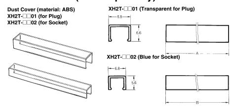
Attach these Dust Covers to Connectors that are not in use. They do not protect the Connectors from flux during automated soldering.
