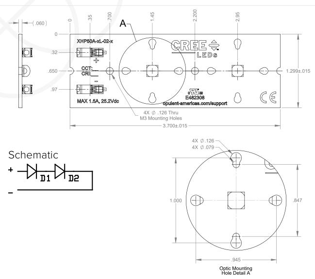
1. Single Poke-In Connectors accept 18-24 AWG solid or stranded wire
