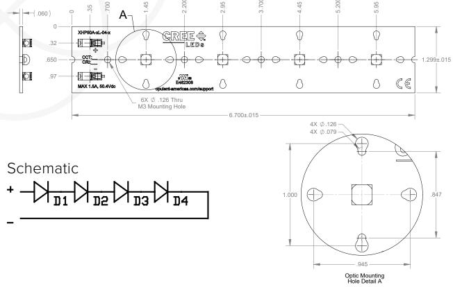
1. Single Poke-In Connectors accept 18-24 AWG solid or stranded wire
