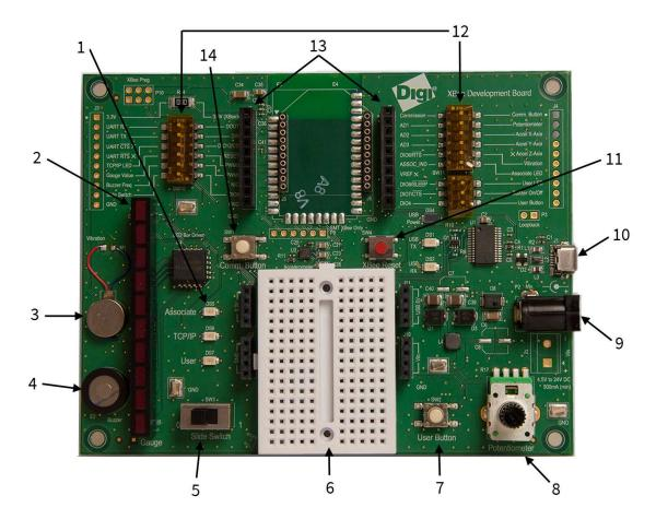
The following table provides descriptions of the XBee Wi-Fi development board components.
