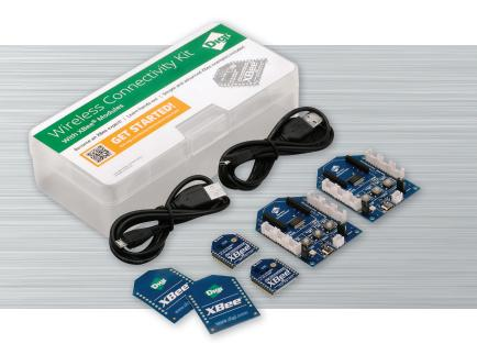
Digi's Wireless Connectivity Kit provides a hands-on way to learn how to use XBee® RF modules for device connectivity and sensor networking.
