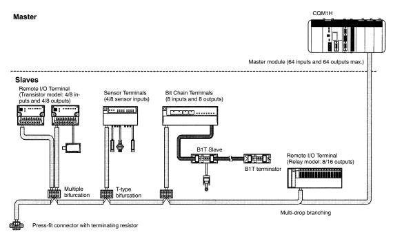
Note: For details about CompoBus/S, refer to the CompoBus/S section in Omron's Remote I/O and Wiring Solutions Catalog (GC RIO1).
