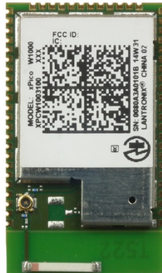
Figure 2: xPico W1003 (XPC W1003) Embedded Device Server
