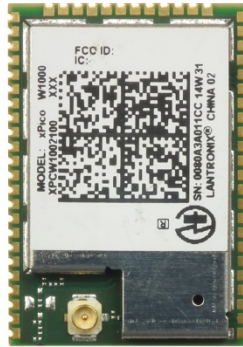
Figure 2: xPico W1003 (XPC W1003) Embedded Device Server
