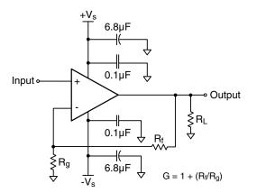
Figure 1: Typical Non-Inverting Gain Circuit
