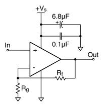
Figure 4: Single Supply Non-Inverting Gain Circuit
