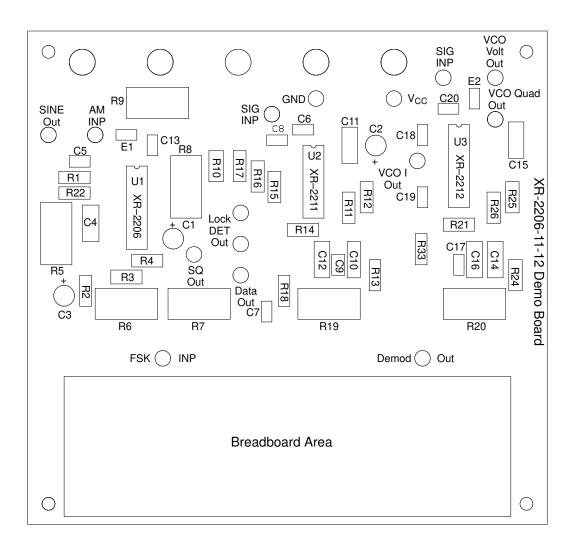
Figure 1. Demo Board Component Layout
