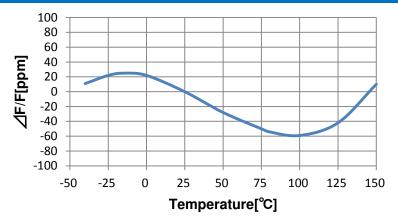
XThis graph shows the frequency shift by temperature of XRCHA16M000F0A01R0
