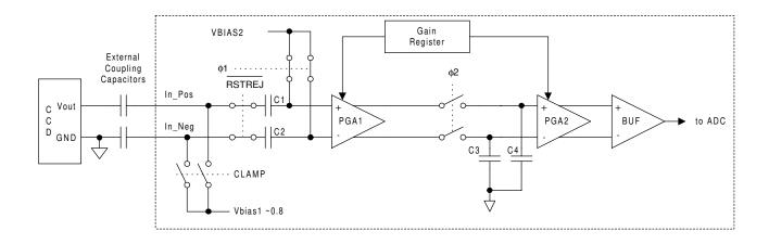
Figure 8. CDS - Black Reference Phase: RSTREJ and \$1 Switch Closed
