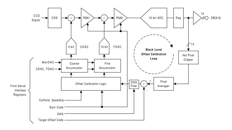
Figure 15. Black Level Offset Calibration Block Diagram
