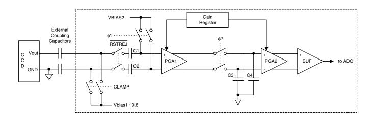
Figure 7. Block Diagram of the CDS, Reset Phase: RSTREJ Switch is Open
