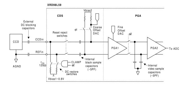
Figure 5. Block Diagram of CDS and PGAs
