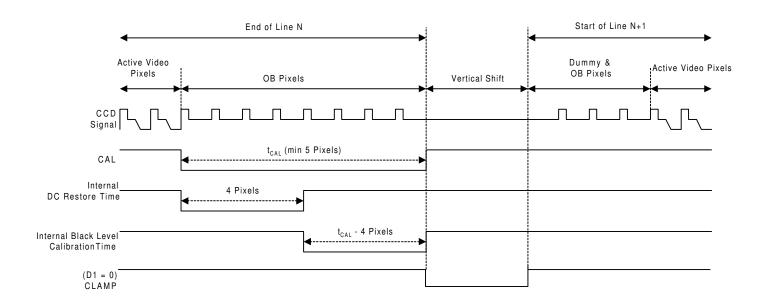
Figure 13a. Example of Vertical Shift Reject Timing using the CLAMP input while in "CAL ONLY" Line Calibration Mode. (CAL and CLAMP Polarity are Serial Port Programmable)
