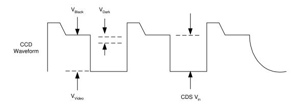
Figure 2. Definition of terms for V  $_{\rm Out}$  of the CCD waveform: CDSV  $_{\rm IN}$  = (V  $_{\rm Black}$  - V  $_{\rm Video}$ )
