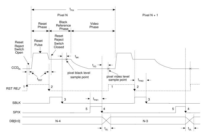
Figure 6. CDS Timing Diagram - Proper Placement of Timing is Critical to Image Quality, SDI=0011 0100 1100
