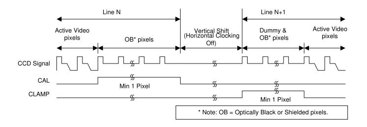
Figure 12. Example of CLAMP & CAL Line Calibration Mode Timing (CAL and CLAMP Polarity are Serial Port Programmable)
