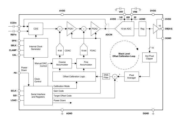
Figure 1. XRD98L59 Block Diagram
