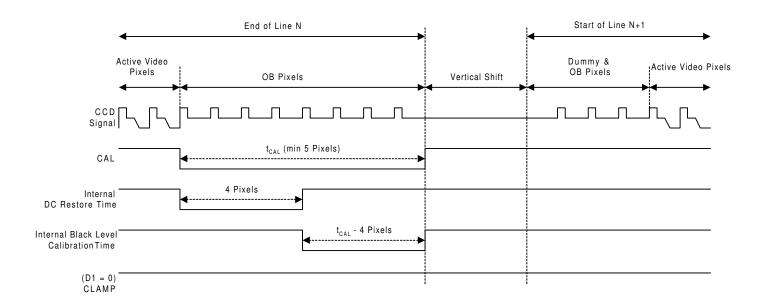
Figure 13. Example of Minimum Timing Requirements for CAL Only Line Calibration Mode (CAL and CLAMP Polarity are Serial Port Programmable)
