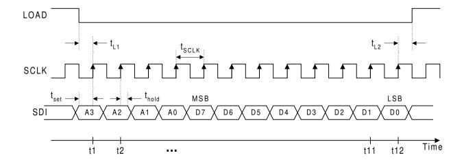
Figure 3. Serial Interface Timing Diagram
