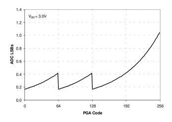
Figure 16. XRD98L59 Offset DAC Step Size in ADC Output LSBs
