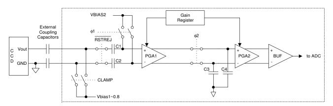
Figure 9. CDS - Video Phase: \$\phi1\$ Switches Open, \$\phi2\$ and RSTREJ Switches Closed
