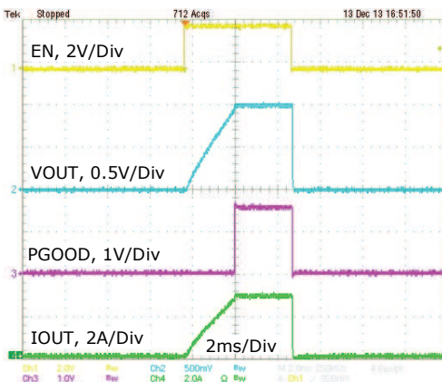
Fig. 11: Enable turn on/off, 3A, 1.5VIN, 1VOUT
