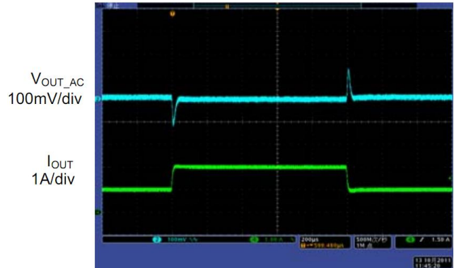
Fig. 11: Load transient ( I_{OUT}=1A to 2A ) Base Time 200\mu s/div
