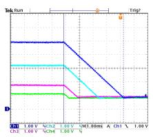
Fig. 16: Sequential Soft-stop V<sub>OUT</sub> Shutdown=0.8V, 3A load CH1:3.3V, CH2:5V, CH3:1V, CH4:1.8V
