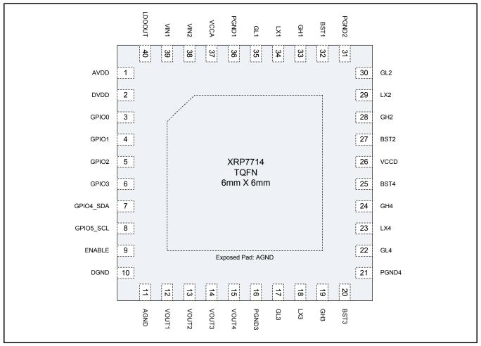
Fig. 3: XRP7714 Pin Assignment
