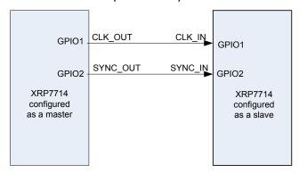
Fig. 28: Master/Slave Configuration of the XRP7714
