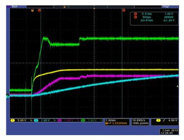
Fig. 22: VCCA (green) Startup Waveform
