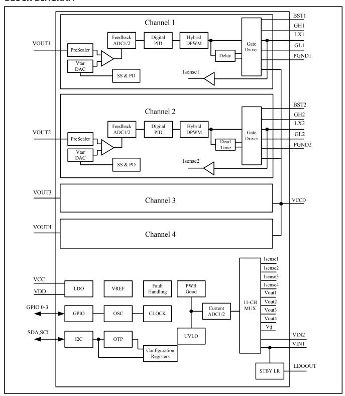
Fig. 2: XRP7714 Block Diagram
