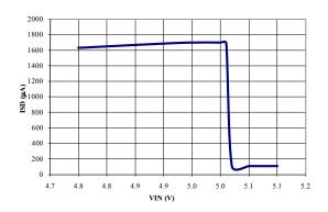
Fig. 11: Shutdown Current 4.8V to 5.1V
