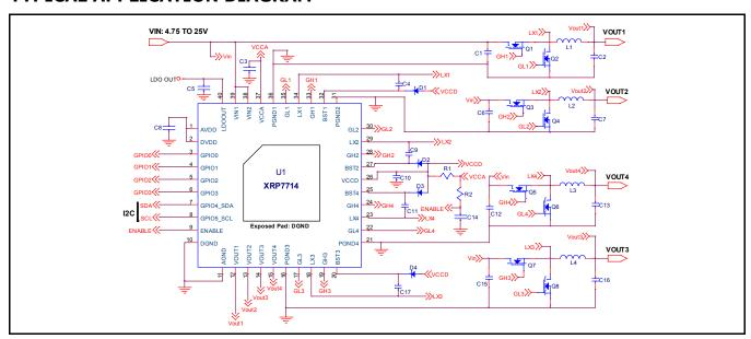
Fig. 1: XRP7714 Application Diagram
