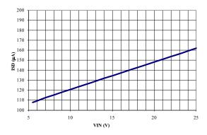
Fig. 10: Shutdown Current 5.1V to 25V
