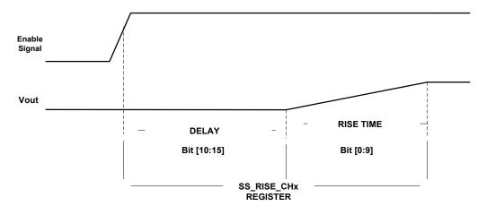
Fig. 24: Channel Power Up Sequence
