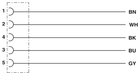
Contact assignment of the M12 socket
