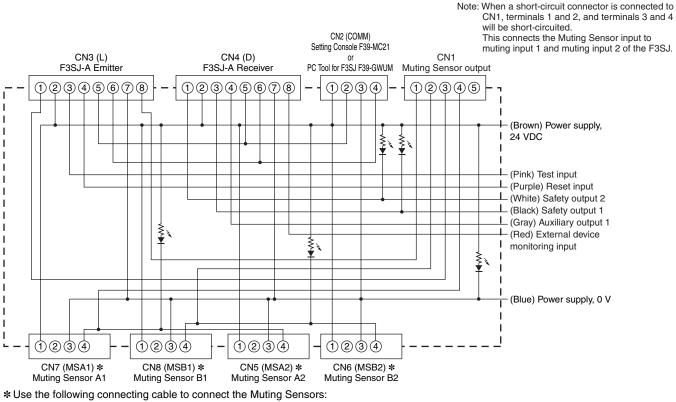
M12, 4-pin connector (Pin 1: +24 V, Pin 2: Not used, Pin 3: 0 V, Pin 4: Output) When using a Through-beam Photoelectric Sensor, use an XS2R-D426-D11-F Y-joint with Socket and Plug or similar product to connect the transmitter and receiver.
