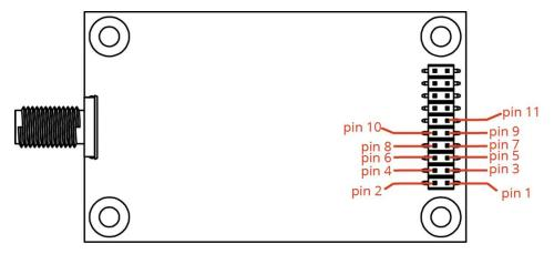
When integrating the module with a Host PC board, all lines not used should be left disconnected (floating).
