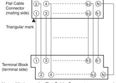
Note: All pins on the Flat Cable Connector correspond 1-to-1 to the terminal of the same number on the terminal block as shown above.
