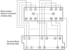
Note: All pins on the Multi-pole, Square Connector correspond 1-to-1 to the terminal of the same number on the terminal block as shown above.
